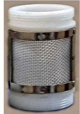
screw type detachable collection bucket Phyto Plankton Net
