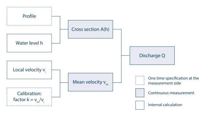
Discharge - The discharge Q is determined by the continuity equation
