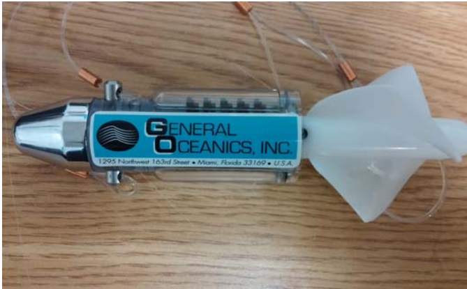
Model 2030R Mechanical Flowmeter With High-speed Impeller
