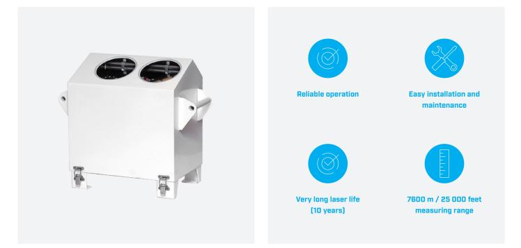
The design is based on the LIDAR principle. The light emitting component is a low power diode laser with the output power limited to an eye-safe level. It is designed for both fixed and mobile installations and detects up to three cloud layers simultaneously.
